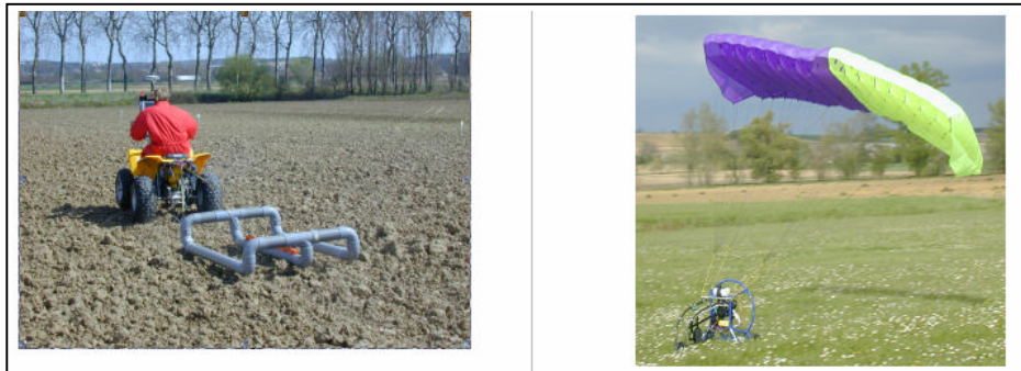
Fig. 2 : EMI EM38 sensor mounted on a 2x4 quad (fig. 2a) and UAV (radio controlled) used for taking spectral image of the fields (fig 2b).
