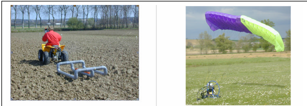
Fig. 2 : EMI EM38 sensor mounted on a 2x4 quad (fig. 2a) and UAV (radio controlled) used for taking spectral images of the fields (fig 2b).
